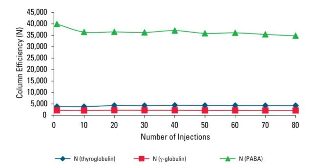
• So the next study was performed with a TSKgel UltraSW Aggregate column from a different lot (W00200-508W) with the use of a guard column prior to the inlet of the column to protect the column from getting fouled.
