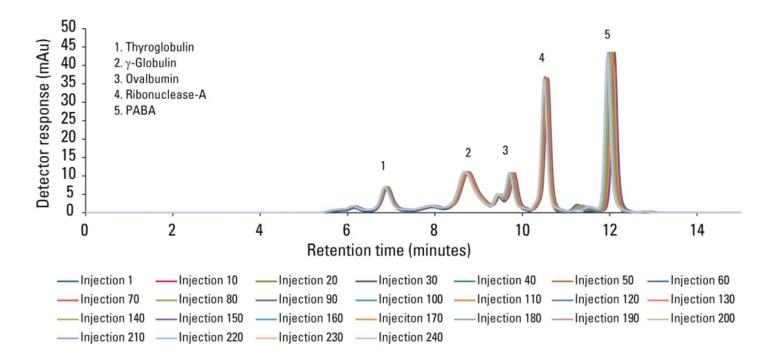
As shown, the chromatograms are reproducible and all of the peak parameters of individual standards are also reproducible.
